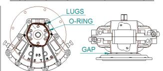
2014 spring housings must be used with 2014 base plates. "Old" spring housings must be used with "old" base plates. Any spring unit can be fitted to any actuator provided the correct seal is used. (see table below)
