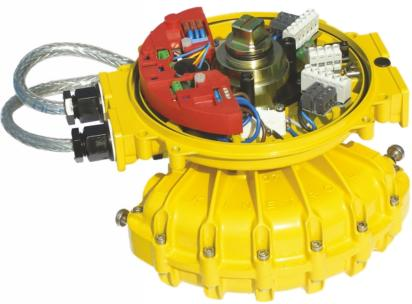
The P3 On/Off positioner consists of an electronic positioning circuit mounted in a robust all-metal enclosure, which controls a ½-turn rotary pneumatic actuator via standard on-off solenoid valves which are direct-mounted on the actuator's own interface.
