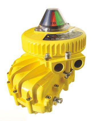
The Explosion Proof Limit Switch Box offers a wide range of signalling options in a compact corrosion resistant aluminium alloy housing. Available for close - mounting onto Kinetrol actuators or discrete mounting via a Kinetrol 05 square or industry standard VDI/VDE interface onto any make of rotary actuator. Easy to wire and set up with true industrial robustness.
