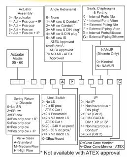
'A' Valve is supplied with all sizes up to and inc' 09 'M' Valve is supplied with 10-15 UNLESS SPECIFICALLY REQUESTED OTHERWISE
