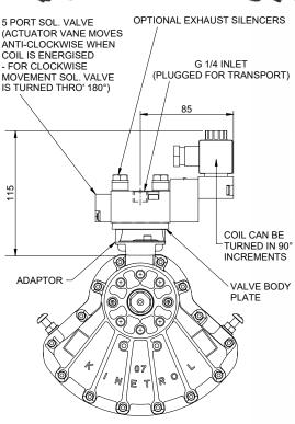
Single solenoid, 3 or 5 port, interchangeable for double acting or spring return, NAMUR interface. Most brands of NAMUR interface solenoid valve can be supplied to special order.
